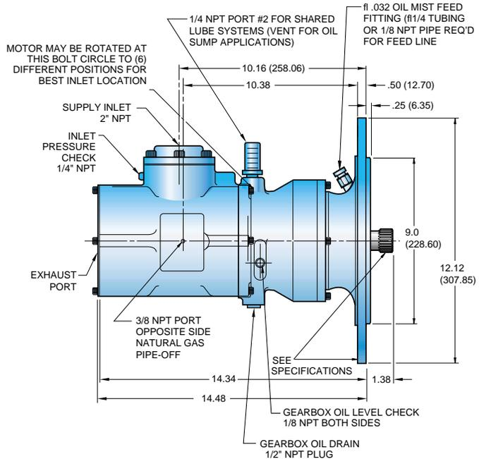
Our Model 56S is designed to mount directly to Solar Saturn engines. An integral soft clutch eliminates the jaw-type clutch assembly, for trouble free operation. And because the 56S motor requires no lubrication in the drive air...fugitive starter exhaust emissions can be totally eliminated.
